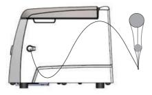
Disconnect the centrifuge from the main supply. Wait until the rotor comes to a stillstand (this may take some time). Once the rotor has stopped, pull out the emergency lid release as
